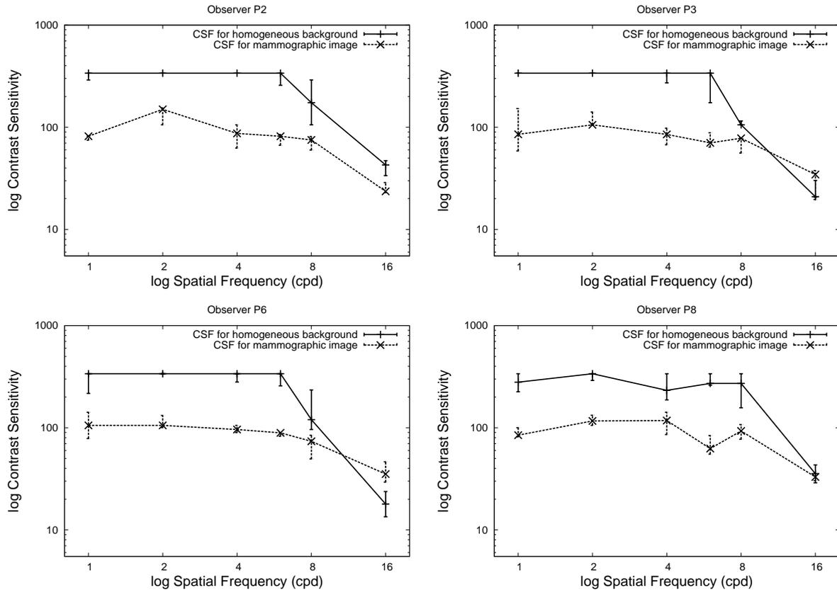
Figure 7. Comparison of contrast sensitivity functions (CSF) acquired with Gabor pattern stimuli on a homogeneous background and a mammographic image, respectively. Results for observers P2, P3, P6 and P8. The difference between the CSF on both types of images is similar for P3 and P6. For the other observers there are stronger individual differences in the shape of both CSFs.
