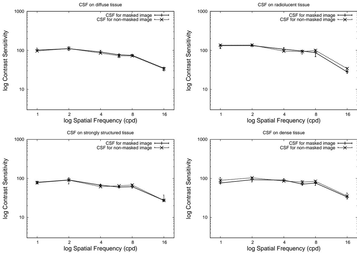
Figure 9. Comparison of contrast sensitivity functions (CSF) acquired with Gabor pattern stimuli for a non-masked and a masked image. Results for measurements performed on the tissues, described in Fig. 5.
