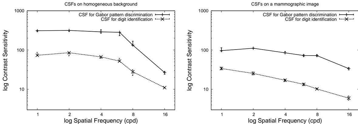
Figure 10. Comparison of contrast sensitivity functions (CSF) acquired with Gabor pattern and digit stimuli, respectively. Results pooled for all observers P1–P8.
