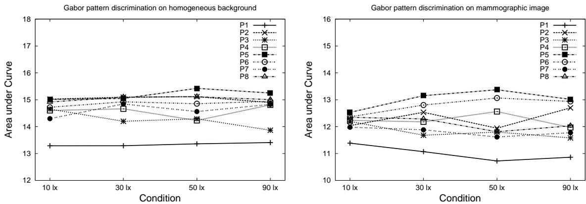
Figure 6. AUC values for the contrast sensitivity functions for all observers P1 – P8 and for the illuminance conditions 10 lx – 90 lx, acquired with Gabor patterns.
