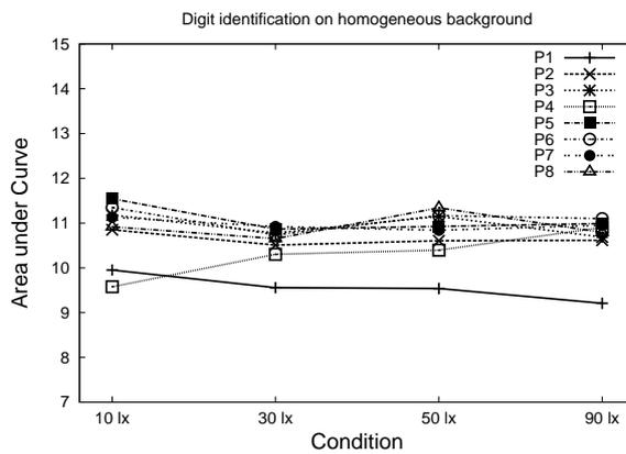
Figure 7. AUC values for the contrast sensitivity functions for all observers P1 – P8, for the illuminance conditions 10 lx – 90 lx, acquired with digits.
