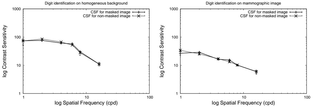
Figure 5. Comparison of contrast sensitivity functions (CSF) acquired with digits as stimuli for a non-masked image to a masked image (data pooled for the eight observers). The behavior is the same as for Gabor patterns, i.e. the contrast sensitivity in the foveal field of view is not improved by the application of a mask. (modified from Apelt et al.<sup>7</sup>)
