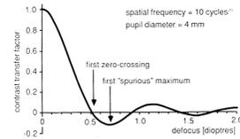
The contrast transfer factor for a defocused periodic sinusoidal grating. At 0.5 D defocus, contrast is zero.
